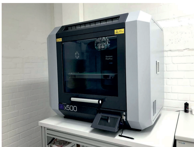
Fig. 1. An FFF printer x500 from RepRap was used to print the examined PEEK samples. © Dennis Prigann, PuK
