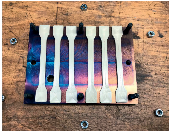
Increasing the degree of crystallization and improving the mechanical properties of 3D-printed PEEK tensile specimens (right) by post-heat treatment in a high-temperature furnace (left). © Dennis Prigann, PuK
